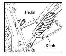
pedal. Slide the pedals forward or backward to the desired position, and then retighten the knobs. Make sure that both pedals are in the same position.
